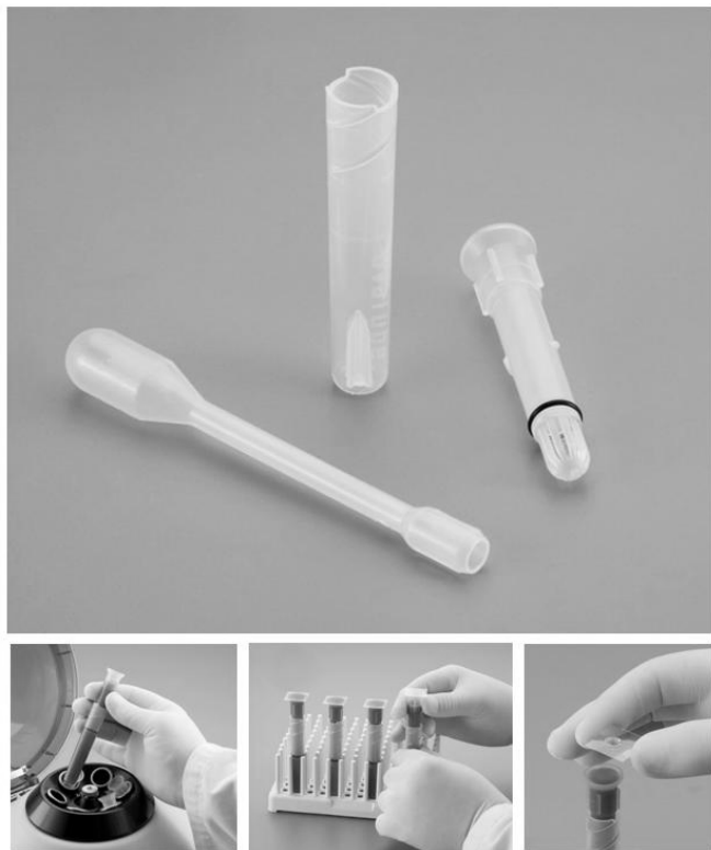
Fig. 1 The StatSpin OvaTube centrifugal flotation device for ova and parasite detection.
